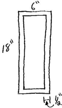
SELF WEIGHT OF CROSS SECTION \* DENSITY OF A36 STEEL =  $0.28 \frac{\text{lb}}{\text{in}^3}$
