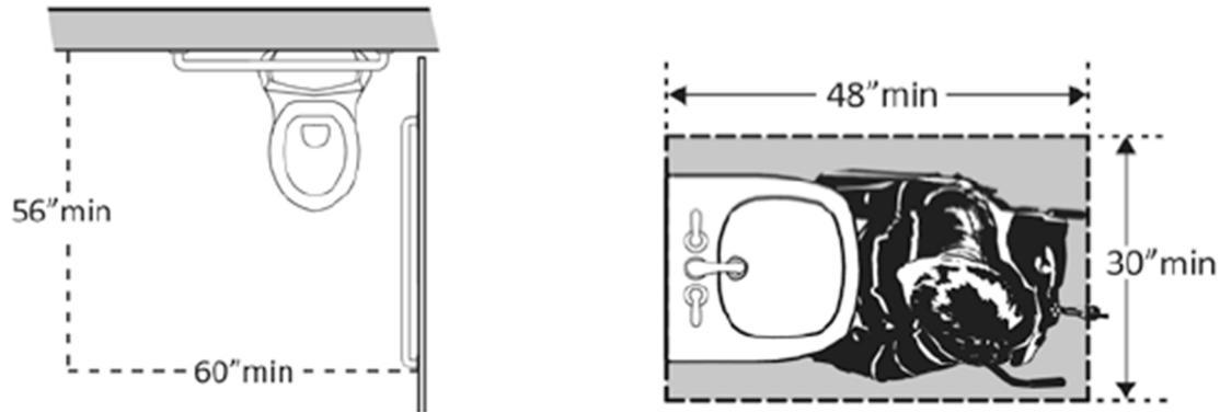
This challenge was overcome by widening the patient restrooms in both rooms. Widening the restrooms created enough space for all of the water fixtures to be placed back-to-back along the same shared wet wall while successfully maintaining ADA compliance. It should be noted that the re-designed restrooms still have a 60" circle of clearance to allow for a wheelchair to turn completely around and maneuver.
