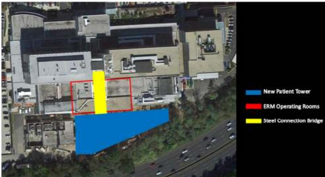
In total this bridge will span 115 feet in length and 16 feet wide for a majority of the bridge. The only portion of the bridge that exceeds 16 feet is the final section connecting to the patient tower. This portion of the bridge, which is 50 feet in length and 23 feet wide, was preassembled by the current project team due to its complex nature and that this section is cantilevering out over the off the patient tower by two
