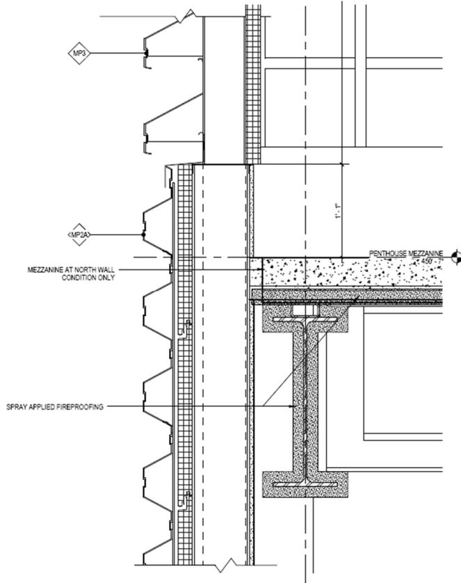
At the mechanical floors located at the top of building, more of a variety of wall types exist. Transitioning from the curtain wall on the sixth floor to the seventh floor mechanical space on the south facing wall, metal louvers clip fasten to 6" louver support framing and receive an insulated blank off panel. The east and west walls at this transition area obtain a 4" corrugated metal panel with fluid applied air barrier, 2" of insulation core material back up panel clip fastened to 8" of
