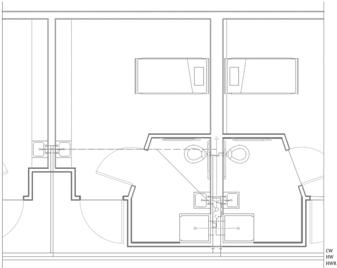
With the relocation of plumbing fixtures and the combining of supplies, sanitary lines, and vents it was necessary to check and potentially resize some of the piping originally specified. To conduct the checking and re-sizing of these pipes the 2009 International Plumbing code was utilized. Through discussions with Adam Davis, a design engineer at Penn State's Office of Physical Plant, it was determined that the sanitary system should be resized first.
